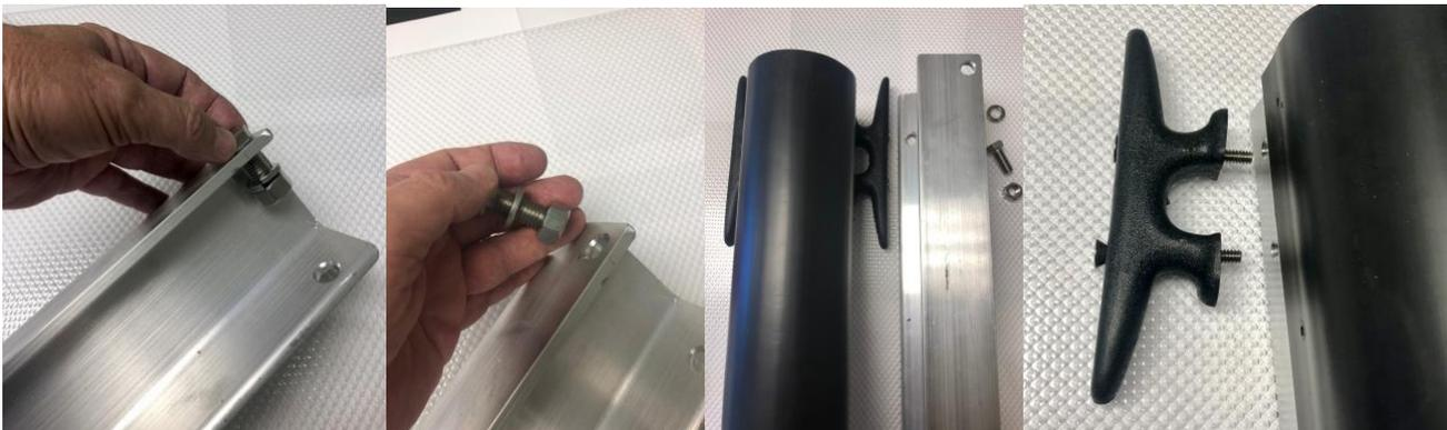
The RatcheTite comes equipped with two ½” stainless steel bolts, lock nuts and spacer plate loosely assembled. Simply remove the two nuts, and place the RatcheTite, spacer and bolts as assembled in the original cleat mounting holes being sure the hex drive fitting is facing up.
