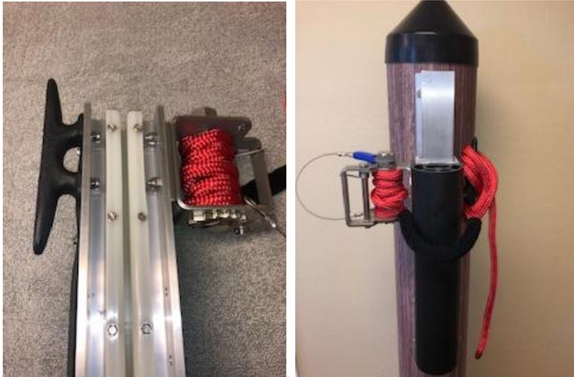
Then insert the tethered tensioning handle on the hex drive and turn the RatcheTite just a few clicks to take up any slack in the line. Do not over tighten the line. Over tightening could damage the cleats on the boat, the cleats on the SlideMoor Slide or the Low Stretch dock Line. Snug is the word!
