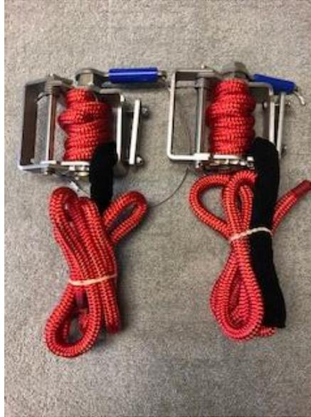
The SlideMoor RatcheTite is designed to end the destructive lateral movement of the vessel while tied to the SlideMoor Docking System due to loose lines. The mechanical advantage provided by the RatcheTite makes that easy. The RatcheTite simply replaces one of the two existing cleats on the SlideMoor Slide.
