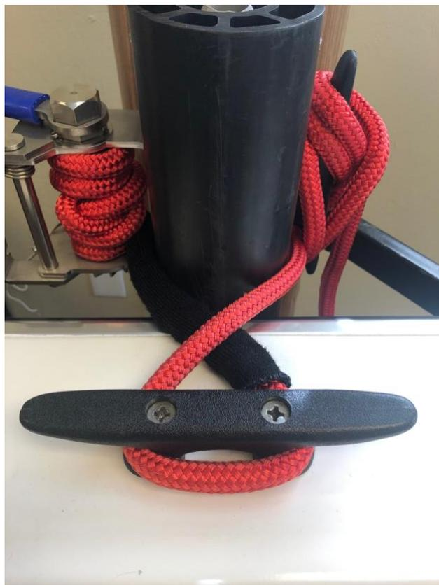
**One wrap and back under the right-side cleat. Pull the slide up while tightening. The line should fairly straight across. The line and sleeve should be coming from the bottom of the coil.**
