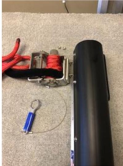
Tighten the two provided ½” stainless bolts and nyloc nuts to the Slide. Be sure to tighten the bolts securely and check their status on a regular basis.
