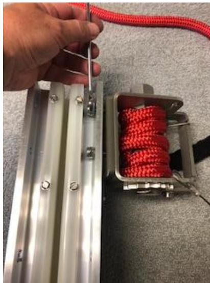
Replace the Slide on the track with the newly installed RatcheTite with the hex drive fitting facing upward and re-secure the track stop bolt. Your RatcheTite is now ready for use.
